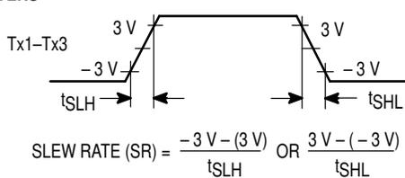
Figure 3. Slew-Rate Characterization
