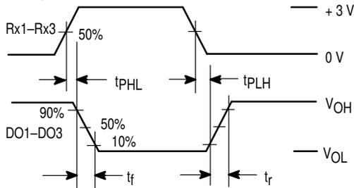
Figure 2. Switching Characteristics
