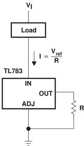
Figure 21. Current-Sinking Regulator
