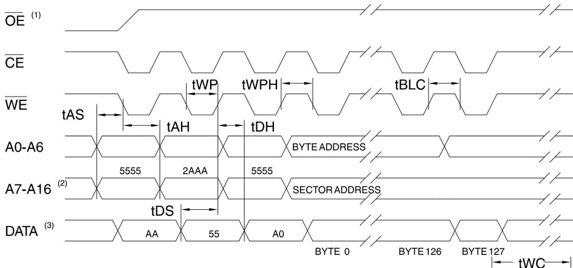
Notes: 1. A7 through A16 must specify the sector address during each high to low transition of  $\overline{WE}$  (or  $\overline{CE}$ ) after the software code has been entered.
